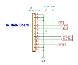
Suggested Mod for J1: Rather than female; the connector should be male since there is not power on these pins when the RF board is not attached to the main board.
